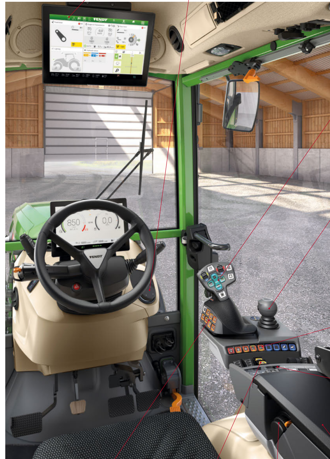
This is where you can easily manage the usual transmission and driving functions with pushbuttons: including two engine speed programs, two cruise control settings and a new dial-controlled active cruise control setting.
